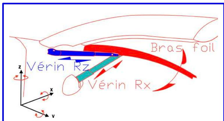
With a  $C_z$  of 1.6, we obtain a foil surface area of  $1.25 \text{ m}^2$  (i.e. an upper chord of 0.8, a lower chord of 0.2 and a wingspan of 2.5 m).
