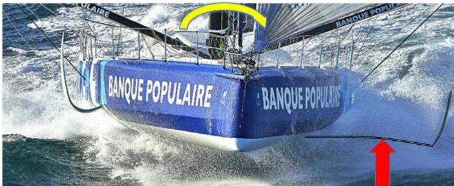
Look at this photo on which I have highlighted the foil, you can imagine that an object (the boat) is pushed up (red line) and that this lift keeps the boat balanced thanks to the capsize moment, while lifting it.
